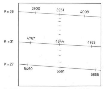
Fig. 3: Schematic of an echelle spectrum. K is the echelle grating order. Wavelengths are shown in Ångströms. Intermediate orders are shown by tick marks. The circumscribed square is the 25 mm  $\times$  25 mm target area of the SEC Vidicon.
