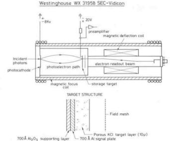
Fig. 2: Schematic drawing of the main parts of a SEC tube.
