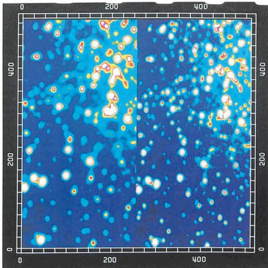
that it was possible to improve the FWHM of the stellar images in long integrations from 0.85 (non-stabilized) to 0.66 (stabilized). The possibility to switch remotely in a few minutes from the f/8 to the f/20 mode was found
