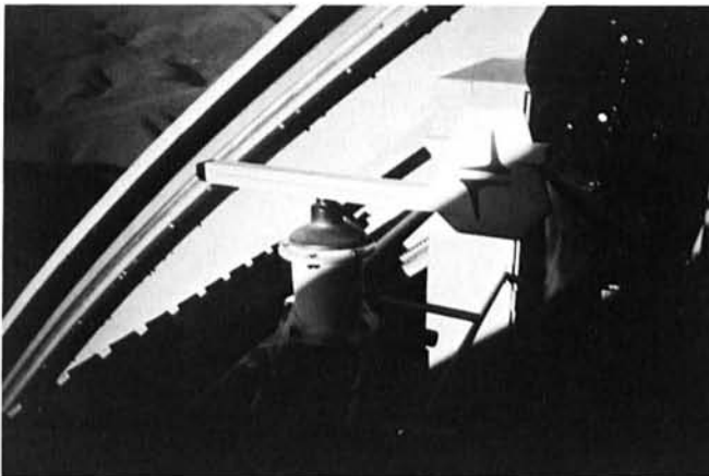
Figure 1: The vortex anemometer placed near the slit (a) and further inside the dome (b).
