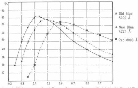
Figure 1: Efficiency curves for (a): The new Blue crossdisperser (filled dots):; (b): The old Blue crossdisperser (filled triangles); (c): The Red crossdisperser (filled squares).
