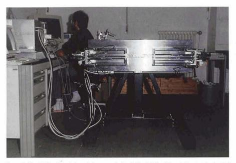
Figure 1: The MOS unit prototype in its support stand. The MOS unit is pointing to a horizontal position. The rack for the control electronics stands on the desk on the left-hand side of the MOS prototype. The tests are operated by a HP workstation in the background of the laboratory. (Photo by M. Pfeiffer, USM.)
