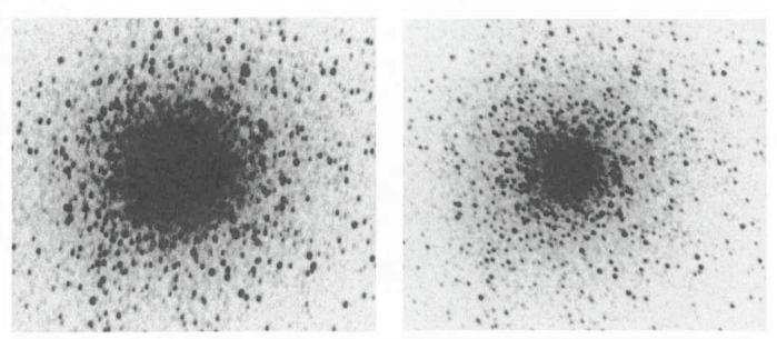
Figure 1: A comparison between the new T-emulsion (right) described in this article, and the ORWO ZU-21 (left) which was much used before. Both photos were obtained by A. Martys with the 50-cm Maksutov telescope at the Crimean field station of the Sternberg Astronomical Institute and show the central part of the globular cluster Messier 13. The photographic reproductions from the original plates were made by H.-H. Heyer at the ESO Headquarters.
