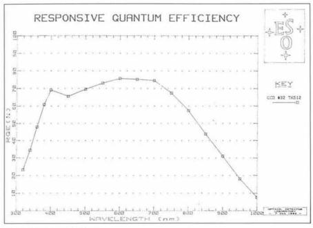
Figure 2: R.Q.E. of CCD #32
