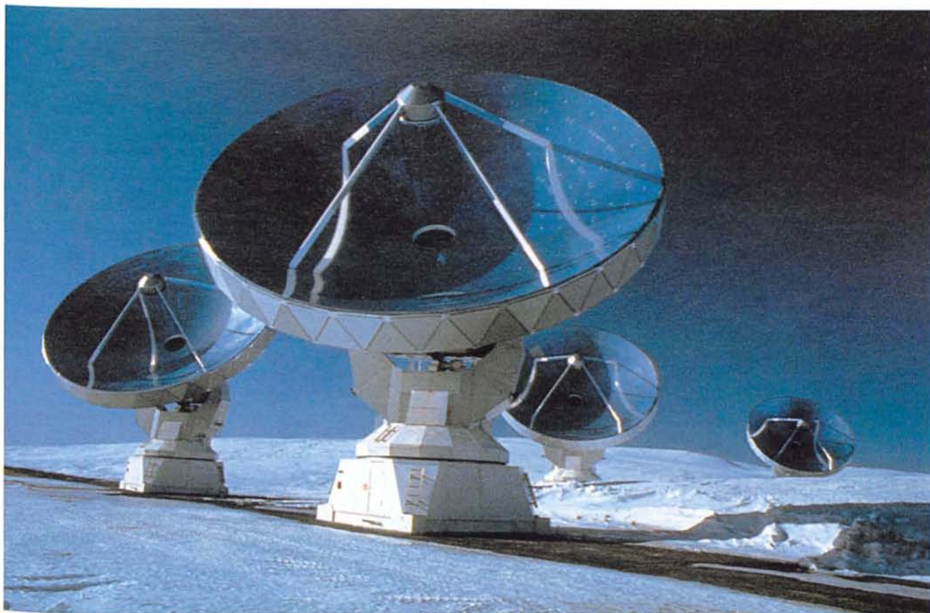
Current state-of-the-art in millimetre arrays: the four 15-m antennas of the IRAM interferometer on Plateau de Bure, France. Photo: A. Rambaud, IRAM.
