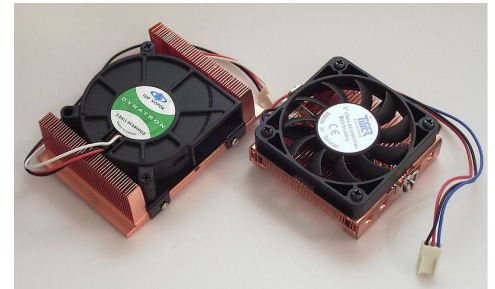
Figure 22 Fans with heat sink mounted for hot spots
