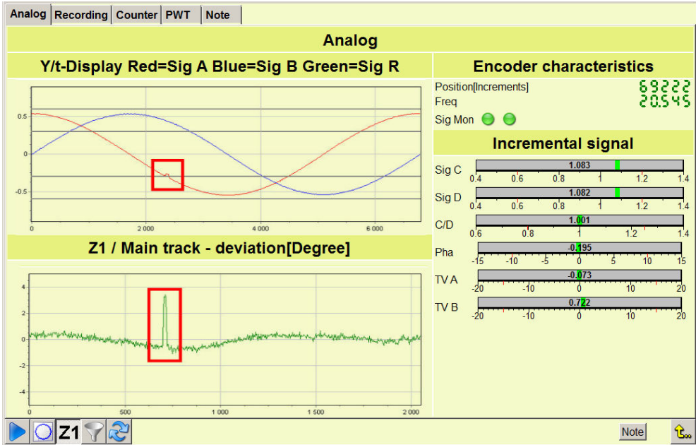
Example: Irregularity (peak) in the sine curve of the commutation signal
