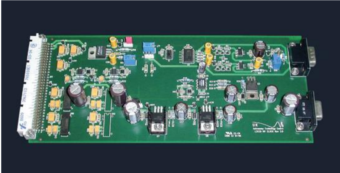
Figure 3 : EMCCD high voltage clock PCB developed for the ASTROCAM controller
