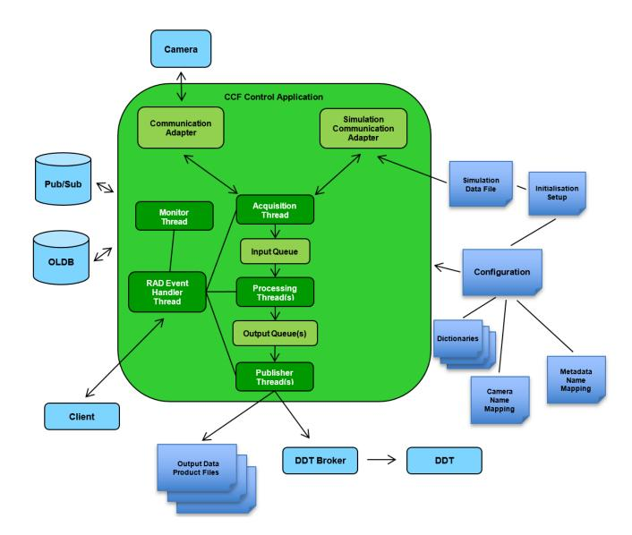
To use the CCF it is not required to have a very detailed/low-level insight into the architecture. Nonetheless, a basic understanding is needed, and useful, to be able to use it and to implement, deploy and test the various adapters needed.
