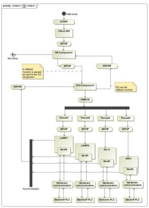
Figure 2: Activity diagram (only ICS part is shown).
