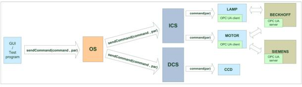
Figure 1: Mock-up prototype software architecture.
