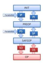
Figure 4: TC3 module state machine (*source: BECKHOFF* website)
