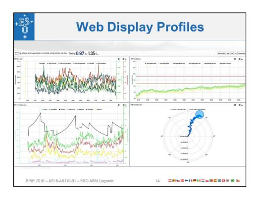
A personal profile with an active warning indication: a wind speed threshold was crossed
