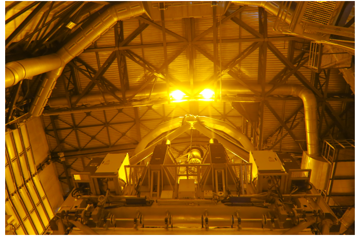
Fig. 3. Picture of the interior of UT4 acquired on 2017-08-15, when the dome was closed, the telescope parked, and all four lasers from the 4LGSF propagated. LGS1 and LGS4 are visible in the picture; their beam hits the cylindrical structure of an air-conditioning duct on the dome roof. The overall glow in the picture is evidence of the high amount of scattering of laser photons by the dome surface. All upper and lower lights in the dome were switched off during the test.
