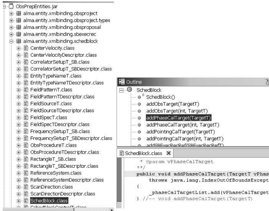
Figure 2. Java XML binding classes generated by the Castor framework, as seen in the Eclipse IDE.
