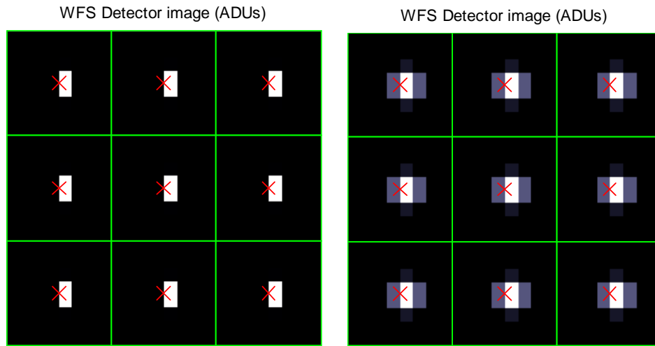
Figure 32: Simulation of 3x3 sub-apertures of MAD under half a pixel tilt, for a diffraction limited source (left) and a source of 3 pixels in FWHM (right).
