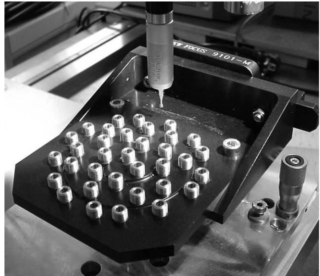
Fig. 4. MAPS entrance plane. Grid of pre-defined positions for plugging the fibers simulating the stars, as designed (left) and during its integration phase (right)
