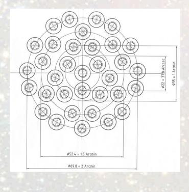
The position of the simulated NGS in the field is defined by plugging the fibres on a mask placed in the entrance focal plane of MAPS. The accuracy of positioning of the NGS will be ensured by the use of standard SMA connector for the fibres end, and their female counterpart on the mask. Those connectors are disposed on concentric rings, and each ring is adjusted in depth in order to simulate the telescope field curvature.
