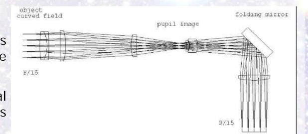
The two groups of optics are manufactured and delivered already mounted in two separate tubes to be attached to the MAPS table. As MAPS shall transfer efficiently from 0.5 to 2.5 µm, the choice of the glasses and coatings was done in order to guarantee high transmission up to IR wavelengths.
