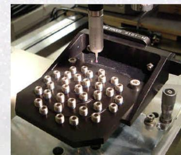
The mask is a metallic plate in which are mounted female SMA connectors. The choice of those standards, easy to plug and unplug connectors allows also changing quickly the configuration of the simulated asterism.
