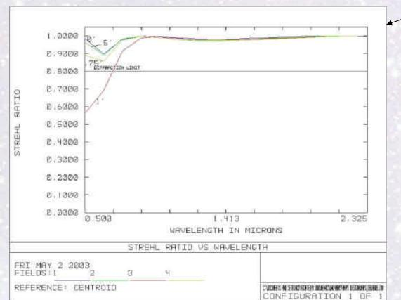
Strehl Ratio performance of MAPS optics up to 1 arcmin from the FoV centre in the spectral range 0.5-2.5 mm, without PSs. A special care was taken when selecting the optics in order to give preference to an excellent and uniform wavefront quality in the IR range (1 to 2.5 µm) to the prejudice of a good quality in the visible. The Strehl Ration in this range is still larger than 55% over the whole FoV, whereas the SR in the IR is fairly constant and never worse than 95%.
