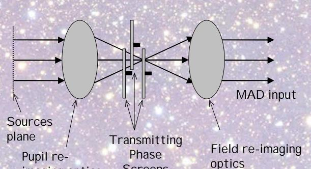
The Natural Guide Stars are simulated by visible-IR light transmitting fibres. A first group of lenses collimates the light beams from the
