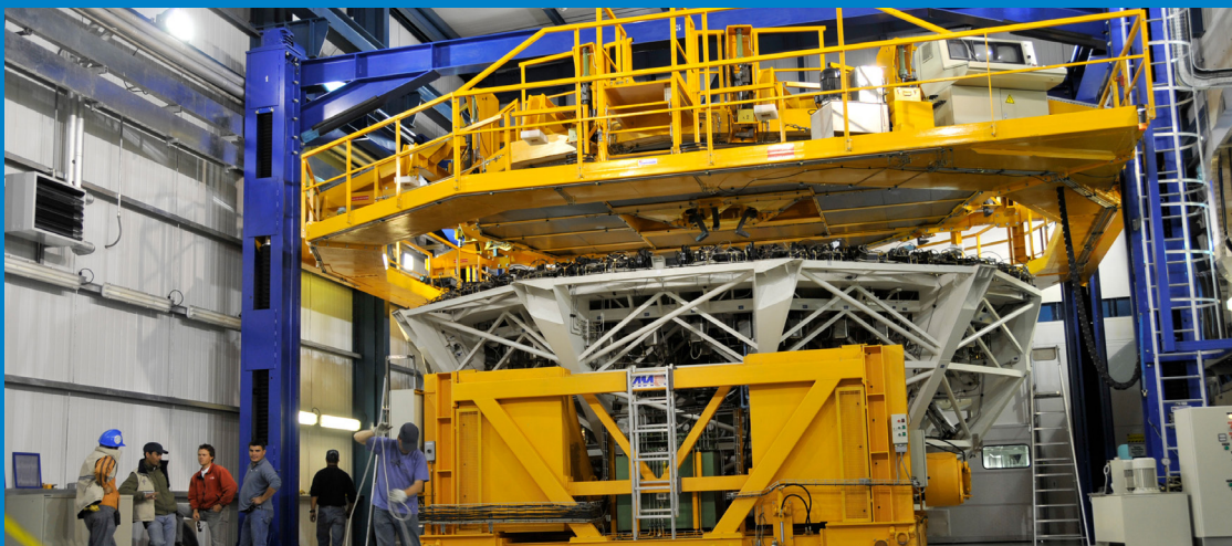
The mirror is removed from its mirror cell by means of a lifting machine.
