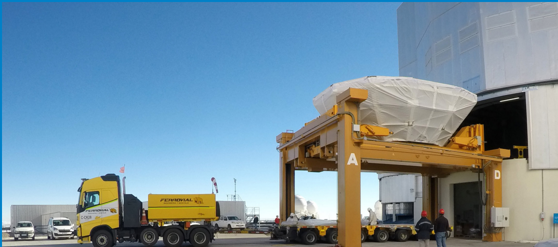
The air cushion vehicle is provided with a lifting device from the telescope and loaded on a special transport truck.
