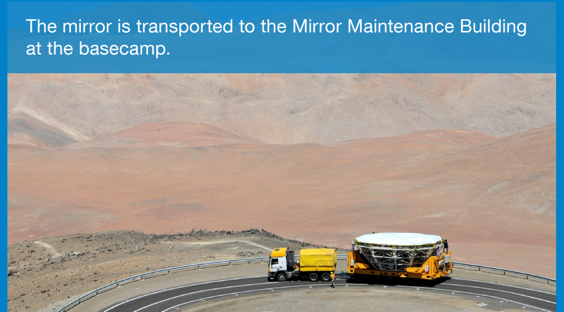
The mirror and its mirror cell (45 ton) is lowered on a special air cushion vehicle.
