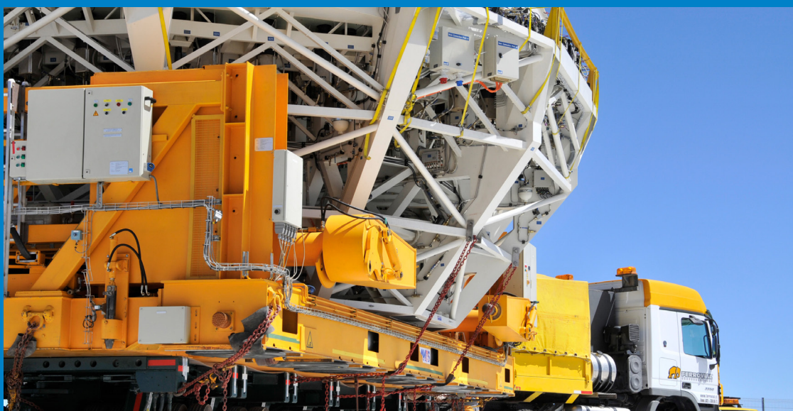
The mirror with the cell is transported back to the telescope.
