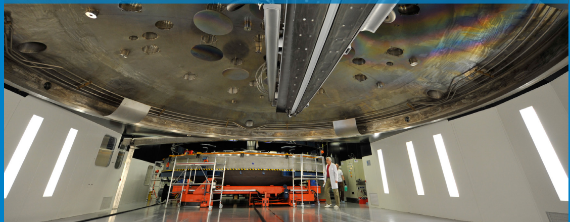
The clean mirror is moved to the vacuum chamber. High vacuum pumps operate an entire night, then a new reflective layer is evaporated with high uniformity during a single mirror rotation by means of cathode sputtering.
