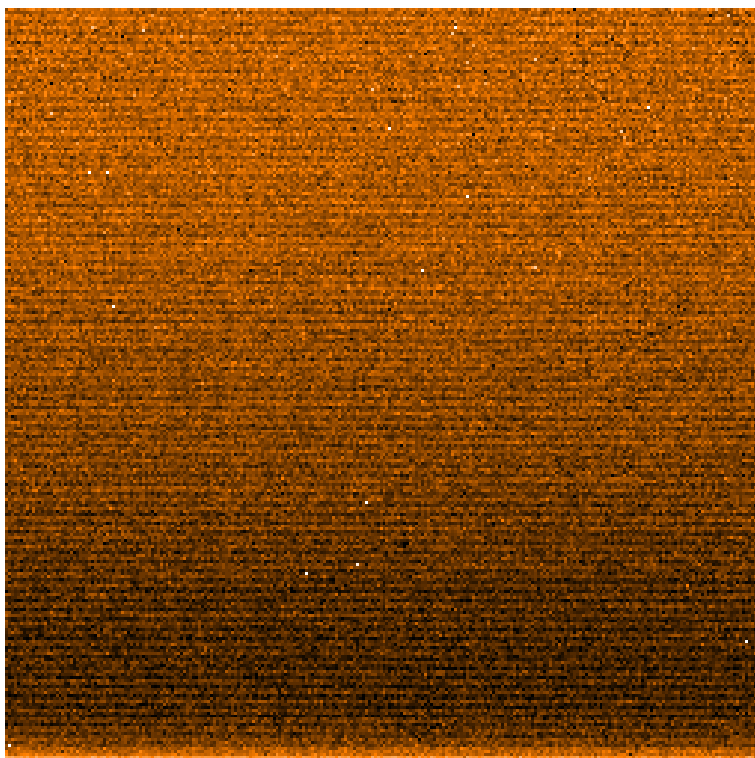
Figure 2: 50 Hz pick-up noise in one quadrant of the Hawaii array.
