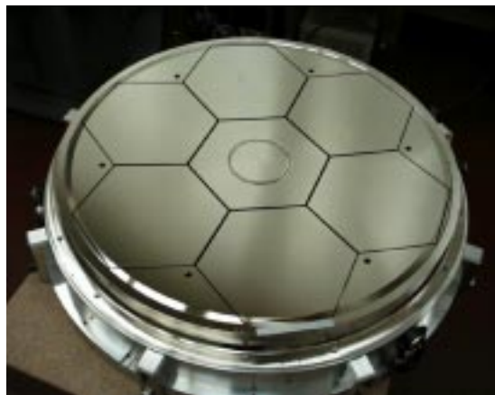
Figure 5.6: The 1 m Segmented DCATT Aluminum Mirror. The mirror figure was provided by Oak Ridge diamond turning. It is being polished at the University of Arizona.
