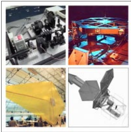
Figure 5.2: Major Testbed and Flight Demonstrations of NGST Technologies. Clockwise from the upper left: The DCATT active optics testbed; the DOTA demonstration of primary mirror deployment; and the Nexus flight demonstration of precision optical control; the ISIS flight demonstration of a deployable sunshade.
