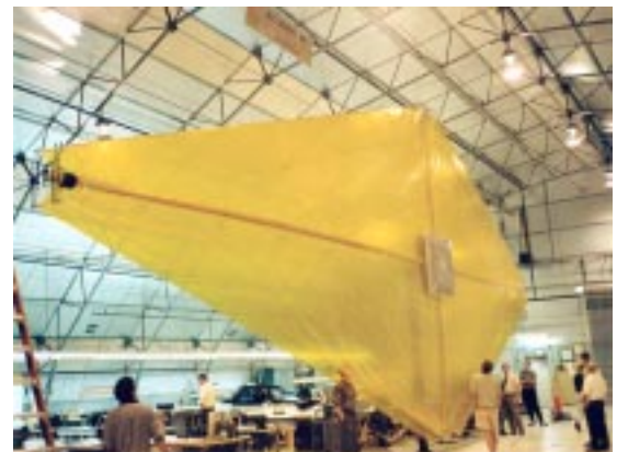
Figure 5.7: The Half-Scale Model of the NGST Sunshield.
