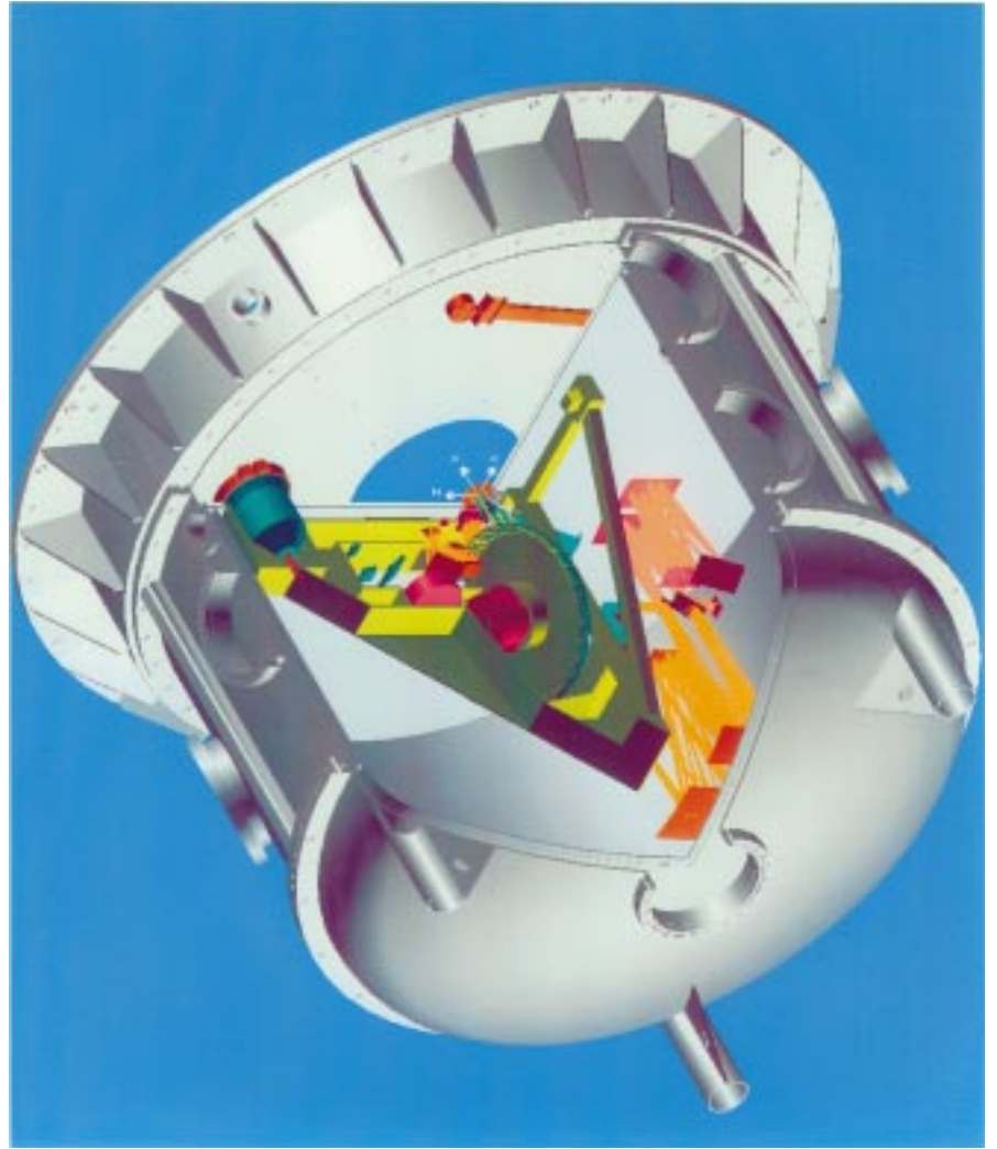
Figure 2: Drawing of the VISIR enclosure, "opened" to show a schematic drawing of the imager mechanical structure. The cryostat is a cylinder of length 0.7 m and diameter 1.2 m. The weight of the cryostat and of the enclosed optical bench is 1 ton. When we consider the total weight of VISIR (cryostat, pumps, cable wrap, electronics boxes ...), we are only 10% below the limit of the VLT unit (2.5 tons).
