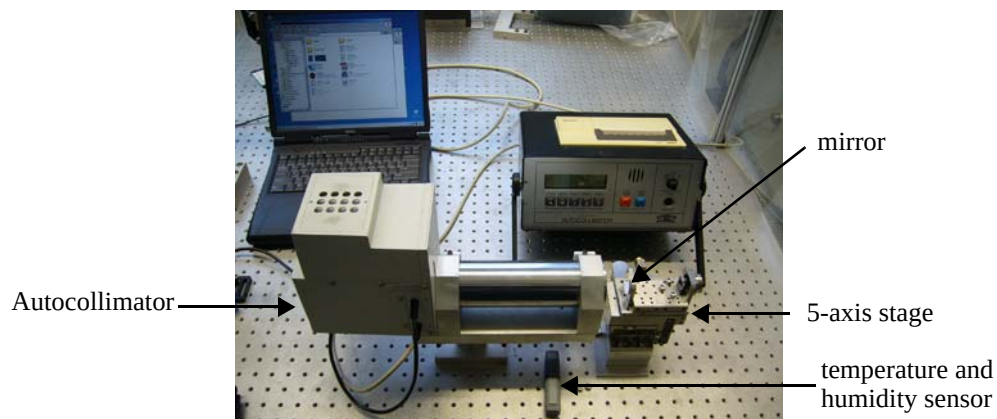
Figure 23 Set-up for the measurement of the tip-tilt created by the 5 axis stage.
