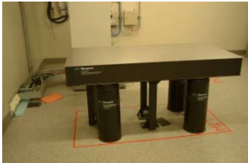
Figure 3 Optical table available at Paranal inside the storage room for the PRIMA Metrology Light source (800x1500mm 2 )
