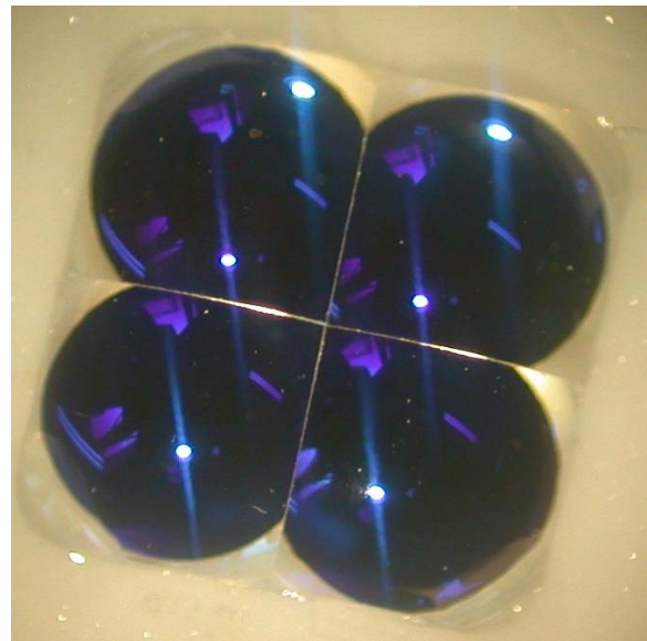
Figure 25: STRAP lens-let array assembly tool, one completed lens-let array
