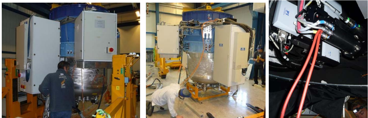
Figure 14: SINFONI maintenance (STRAP Head exchange, right picture)
