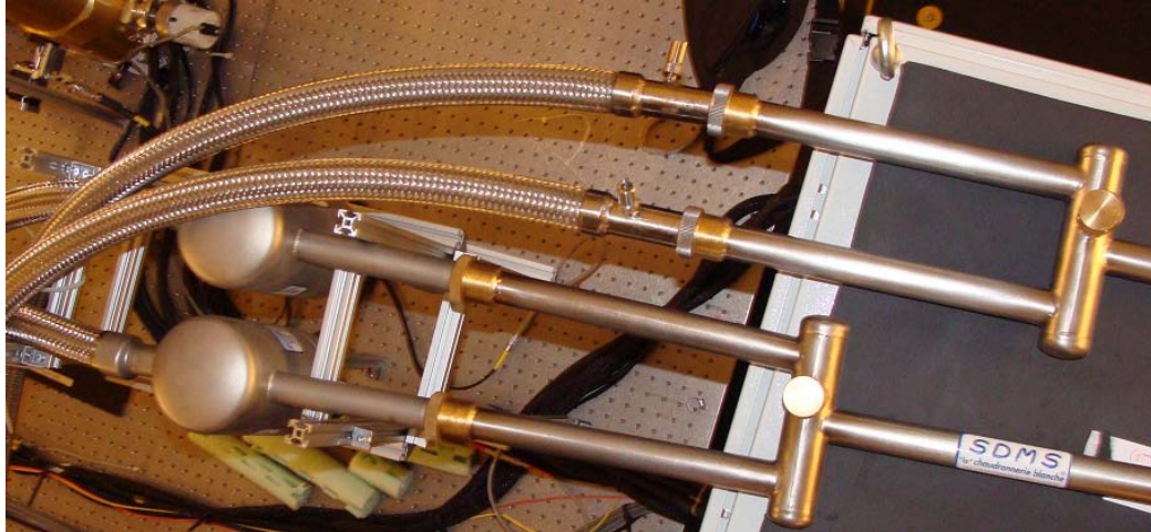
Figure 24: Special connections and lines for the LN2 supply of PIONIER
