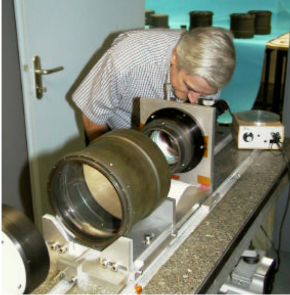
Figure 5: The VIMOS cameras, ( left ) combination CAM+CWL being tested at SESO (Aix, France), ( right ) three of the cameras and CWLs, each camera+barrel weights 30kg.
