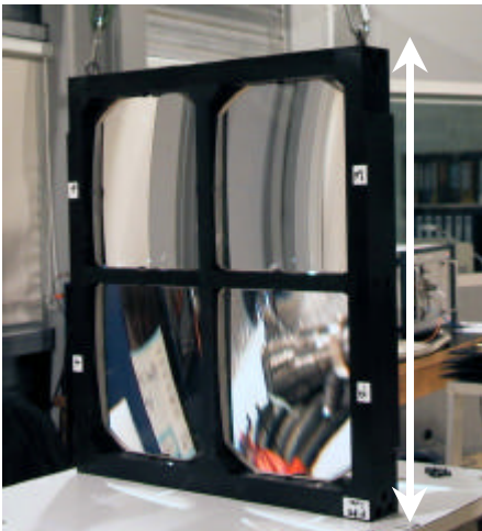
Figure 4: the VIMOS collimator, with the Pupil Relay Lens (left) with overall dimensions 830x760mm, and the 4 last doublets of the collimator in their mounts (right)
