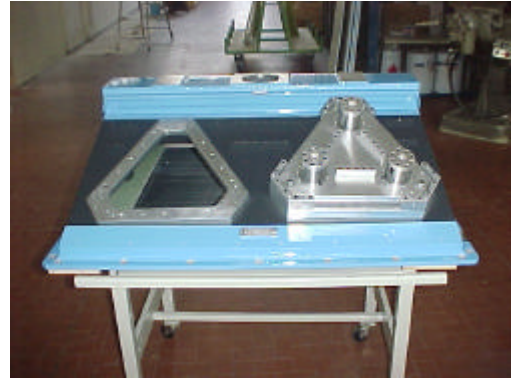
Figure 11: the Folding mirror unit. The 3 cylinders seen on the right are designed to house piezo-actuators for active tip-tilt control of the mirrors
