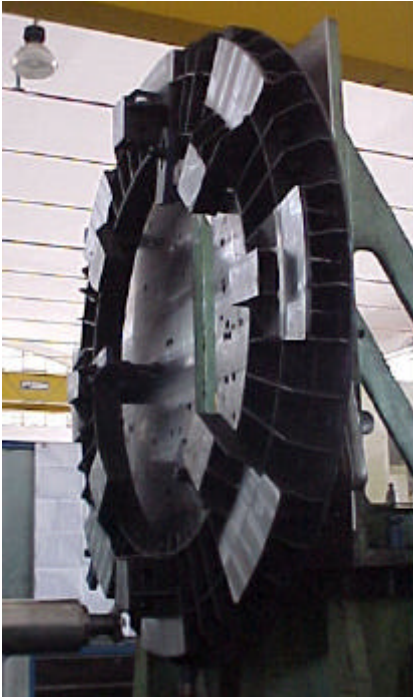
Figure 6: the VIMOS main structure, (left) baseplate interface to the Nasmyth rotator, (right) the main structure serrurier trusses.
