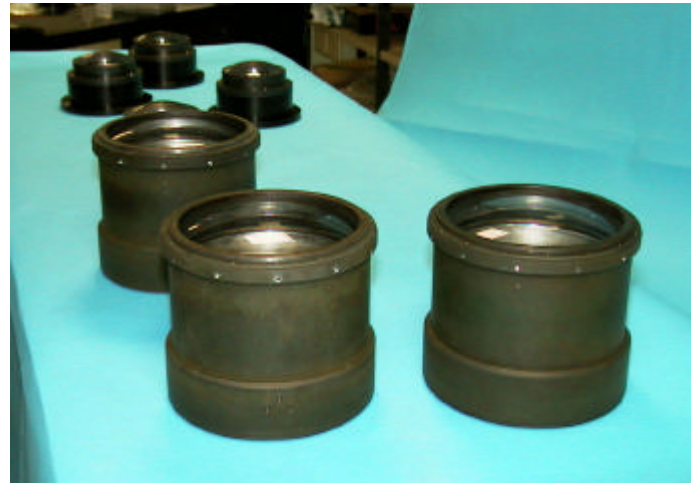
Figure 5: The VIMOS cameras, ( left ) combination CAM+CWL being tested at SESO (Aix, France), ( right ) three of the cameras and CWLs, each camera+barrel weights 30kg.
