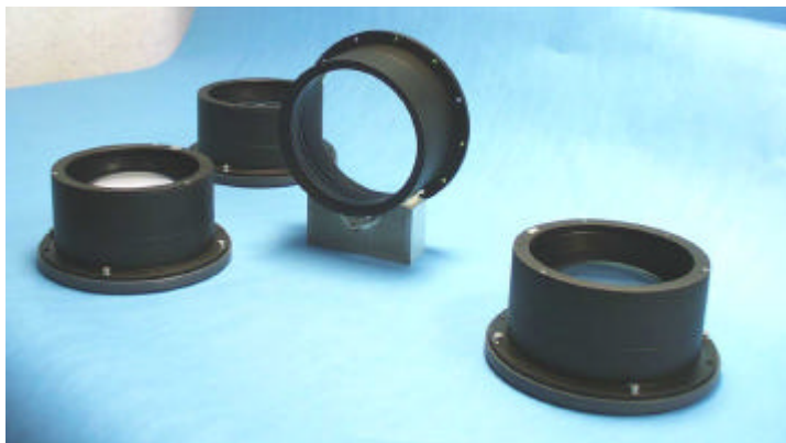
Figure 4: the VIMOS collimator, with the Pupil Relay Lens (left) with overall dimensions 830x760mm, and the 4 last doublets of the collimator in their mounts (right)
