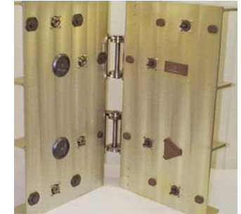
Hinge and Latches Tested for Repeatability
