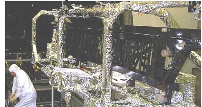
Full-Scale Test Structure (DOTA) Entering XRCF Test Chamber
