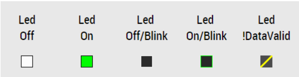
Fig. 5: All possible sates of LedBox Control with default colors
