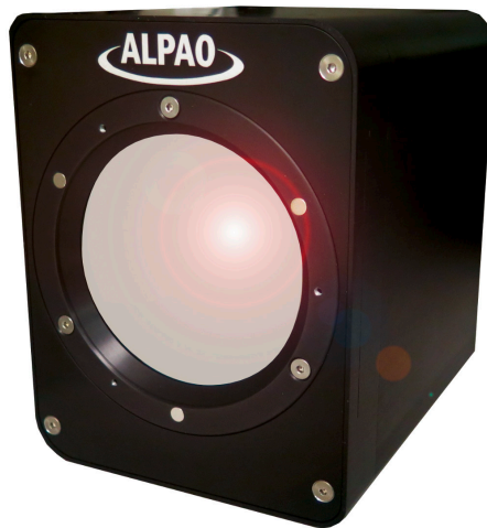
Deformable mirror with 3228 actuators and a 95-mm diameter developed by ALPAO (France) funded under the ESO Technology Development programme; The mirror is currently being used for the validation bench of the ELT instrument MICADO.
