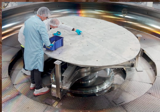
Inspecting mirror samples on the dummy M5 mirror during commissioning of the ELT's Large Coating Plant.
