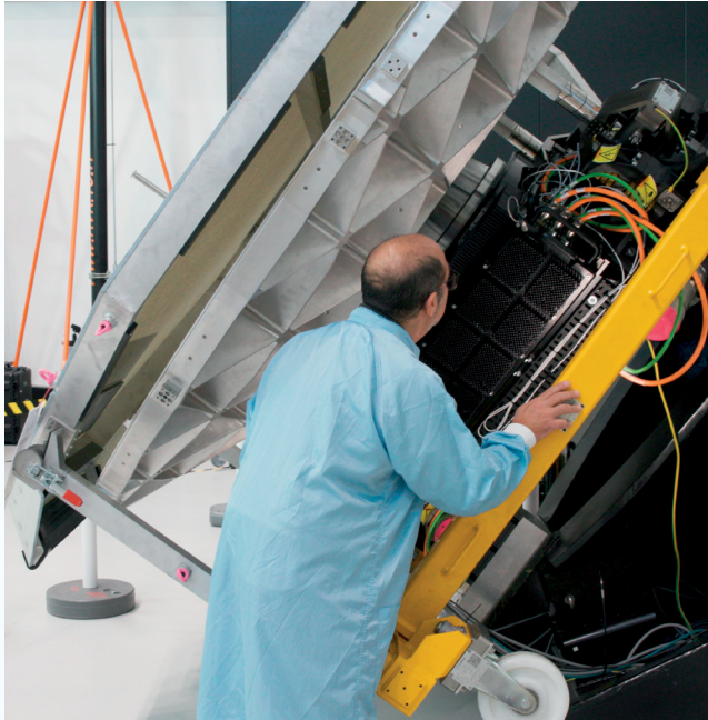
The M5 mirror support cell operating in the Large Integration Hall at ESO Headquarters.
