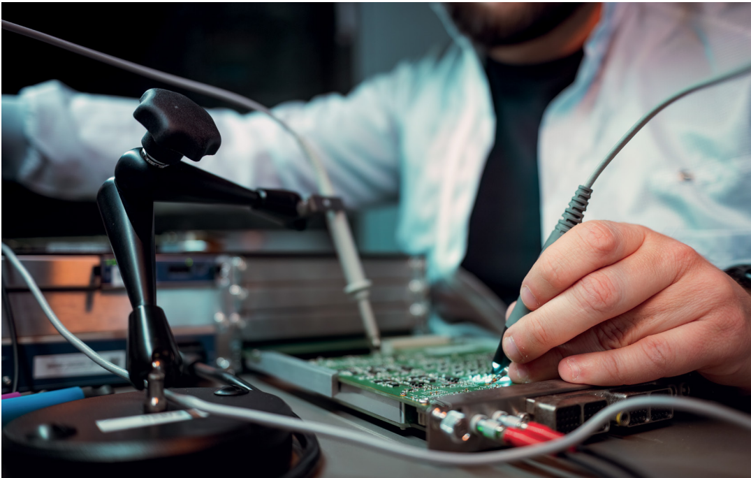
Testing a hardware module for the NGC II detector controller.
