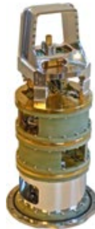
An assembled ALMA Band 5 receiver cartridge.
