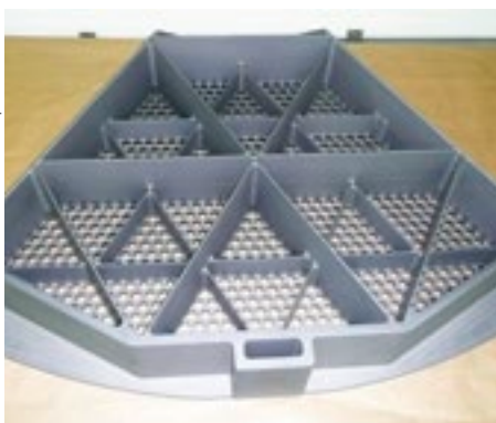
The test version of the silicon carbide M4 support structure.
