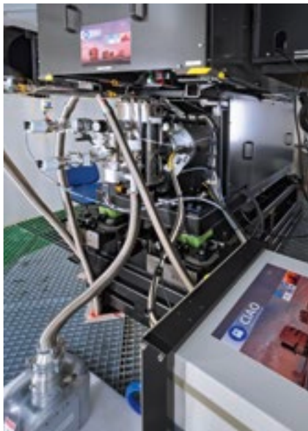
The CIAO infrared adaptive optics Unit 1 in final configuration at VLT Unit Telescope 1.
