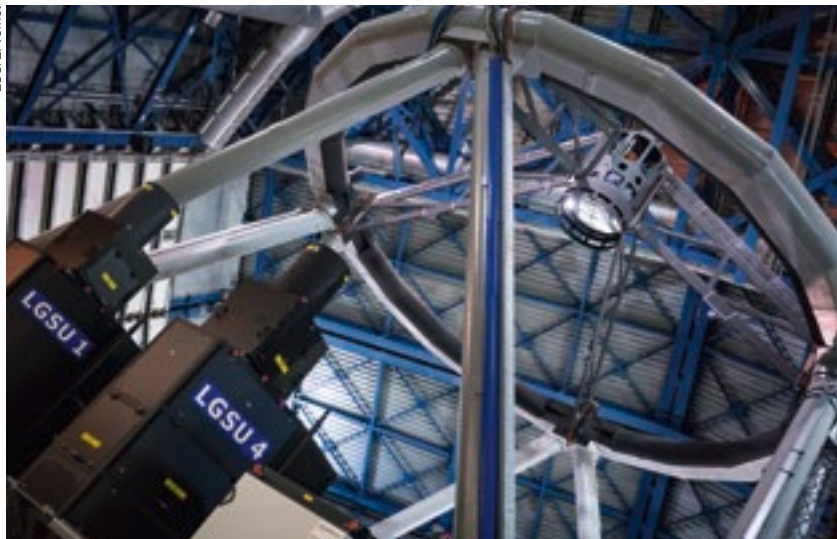
The DSM and two of the four Laser Guide Star Units of the 4LGSF on UT4.
