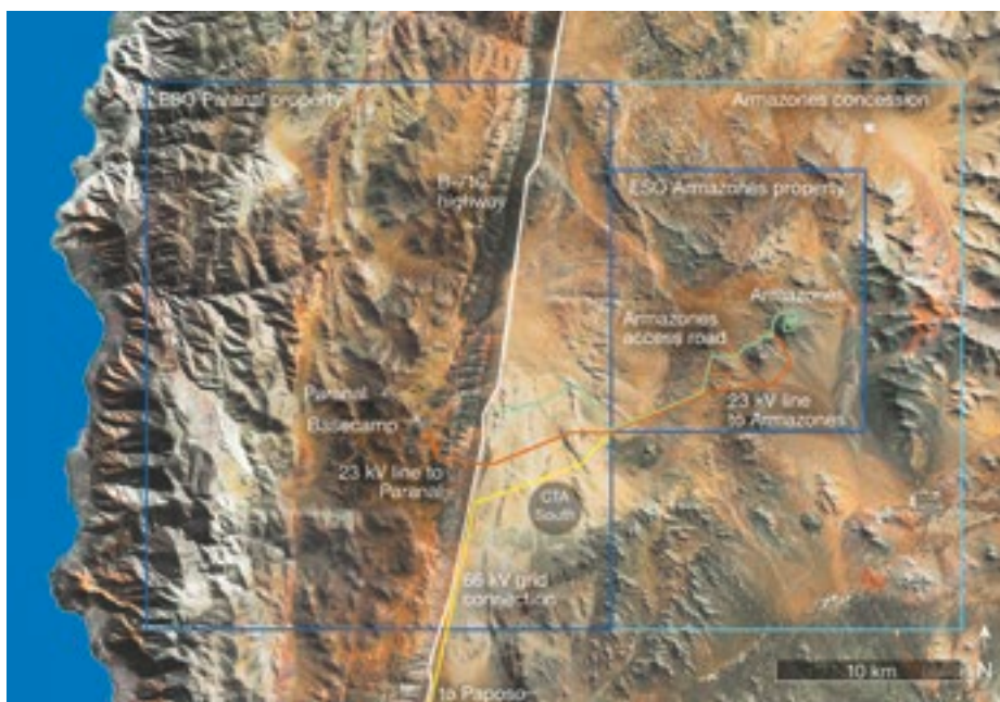
Map of the Paranal Armazones area, showing the planned connections to the Chilean electrical grid.
