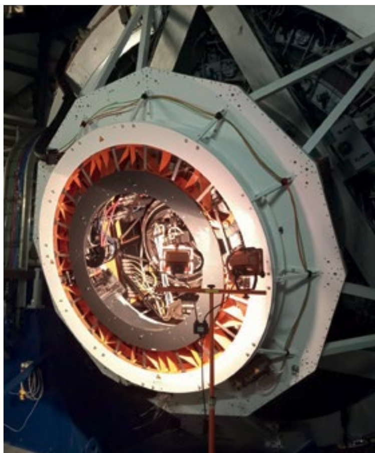
The new cable wrap and adapter-rotator for 4MOST, installed on VISTA.
