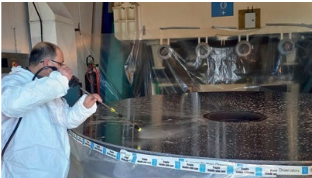
Testing high-pressure washing of the NTT mirror.
