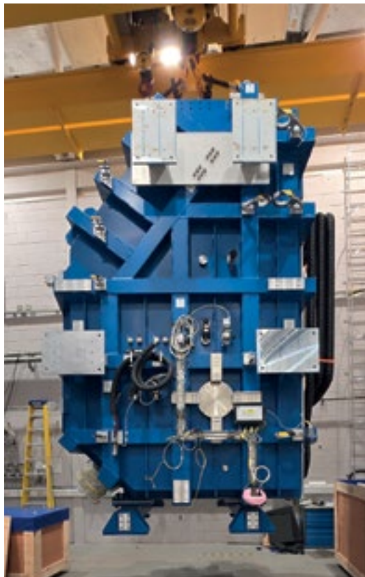
The completed MOONS cryostat, with a mass of 9.5 tonnes, is lifted in December 2025 in preparation for its transport to Chile.
