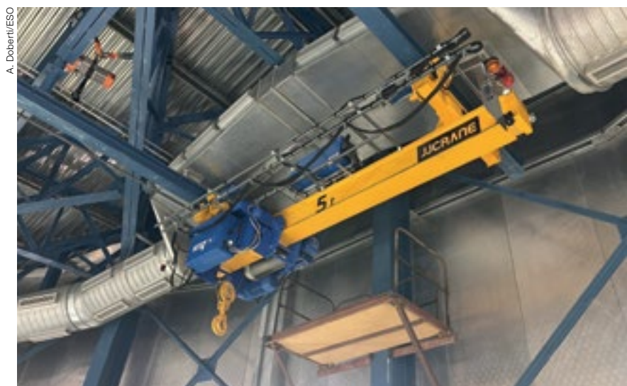
New five-tonne capacity crane installed at the VLT.
