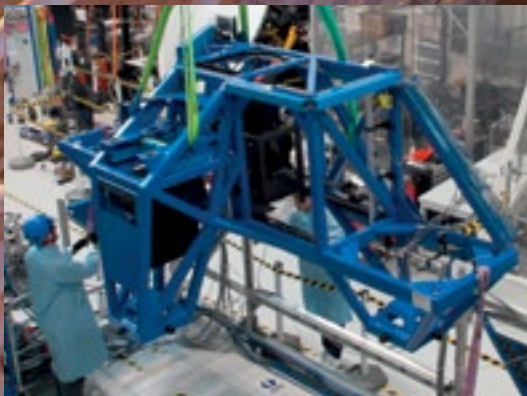
The mechanical structure of the ELT Phasing and Diagnostic Station is lowered into position in the Large Integration Hall at ESO Headquarters.
