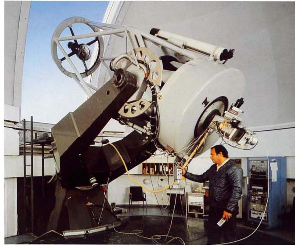
223–224 Two important instruments on the mountain are the 1.5-m spectroscopic (Plate 223) and the 1-m photometric telescope (Plate 224). As the names indicate, they are mainly used for spectroscopy and photometry of stars and galaxies.
