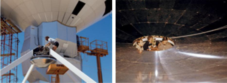
*After the fire. Photo left: Preparing the new subreflector for the SEST. Photo right: Albert Grewe measuring the accuracy of the reflecting panels with a theodolite. (Photos by the author)*
