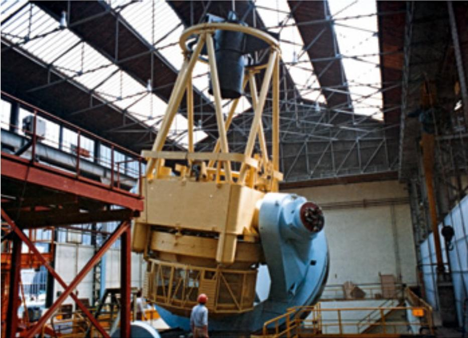
*The main mechanical structure of the 3.6-metre telescope at the factory site of Saint Chamond.*
