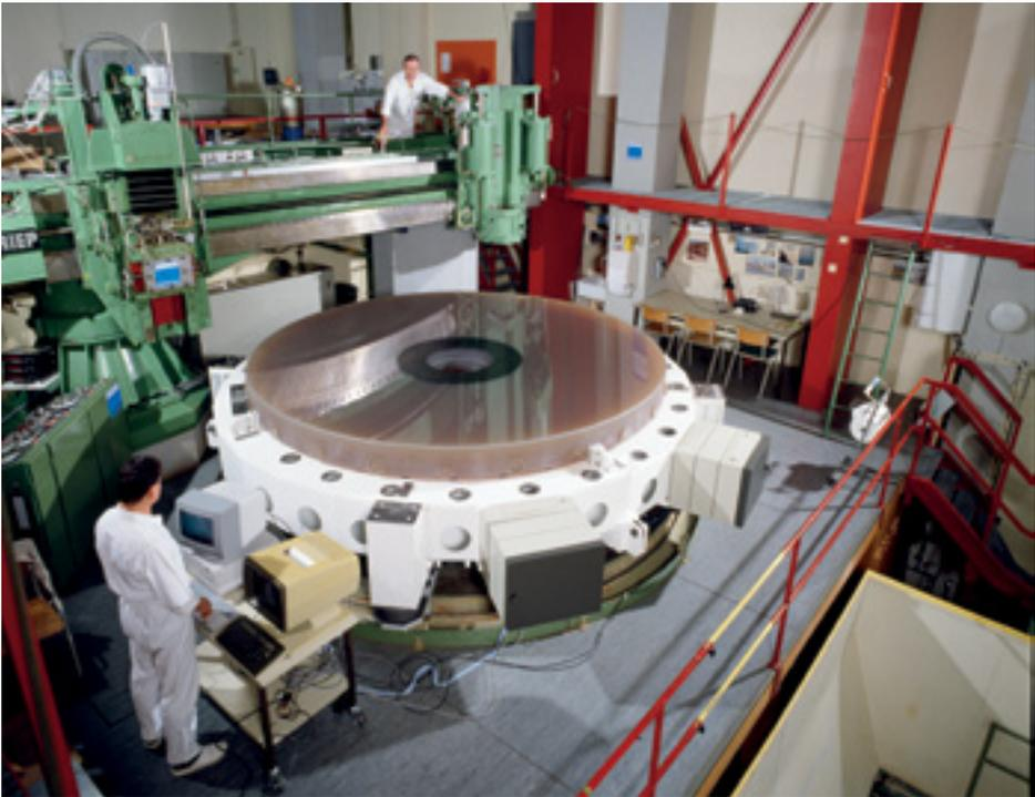
*The NTT primary mirror at Zeiss, mounted on the support structure, seen shortly before delivery to ESO. (Photo by the author)*
