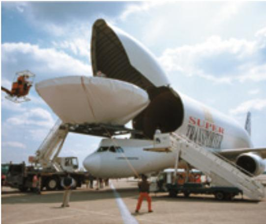
*Loading the prototype antenna into the Airbus Beluga transporter. (Photo: Massimo Tarenghi)*
