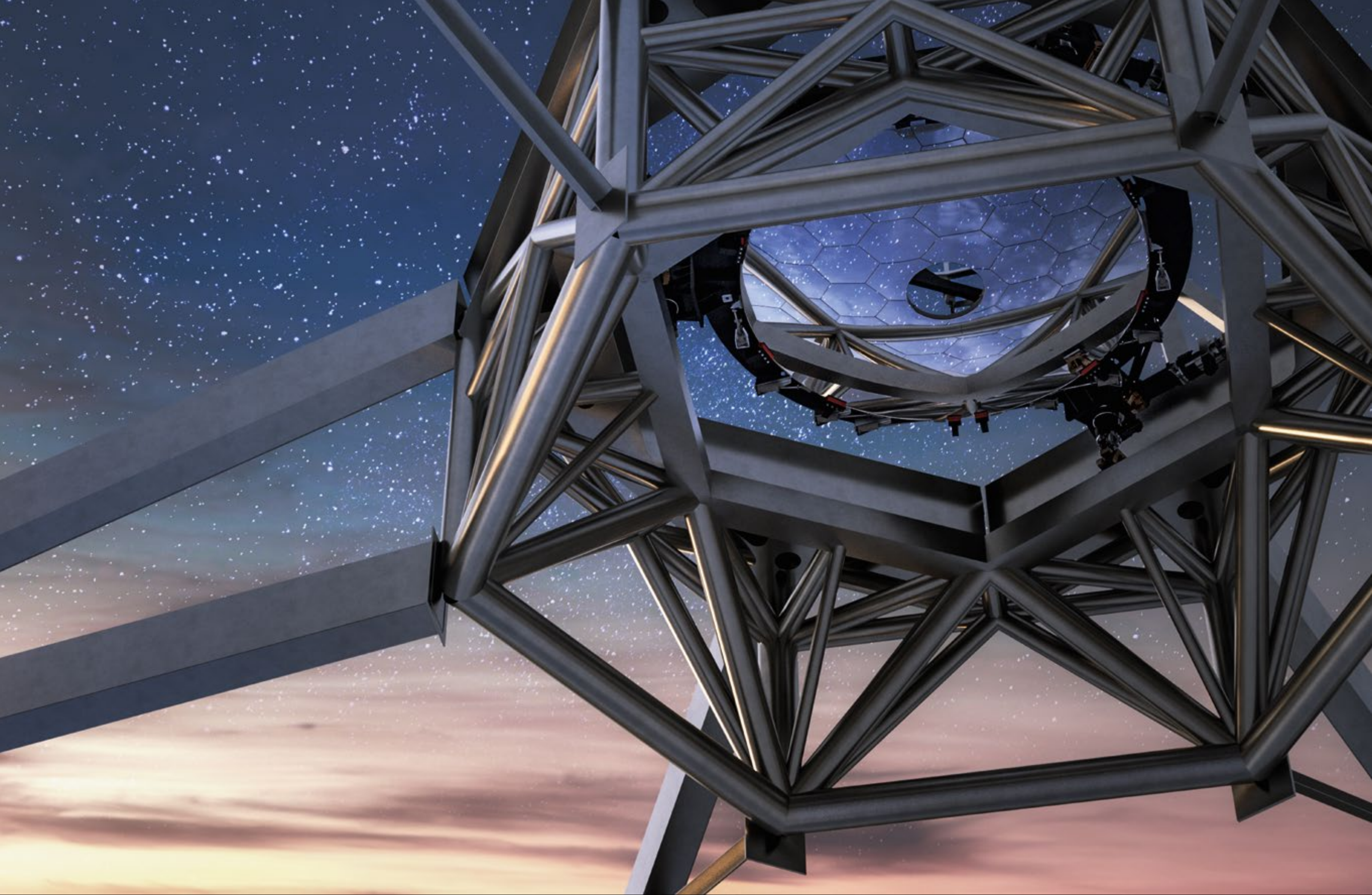
Rendering of the M2 mirror in position on the ELT telescope
