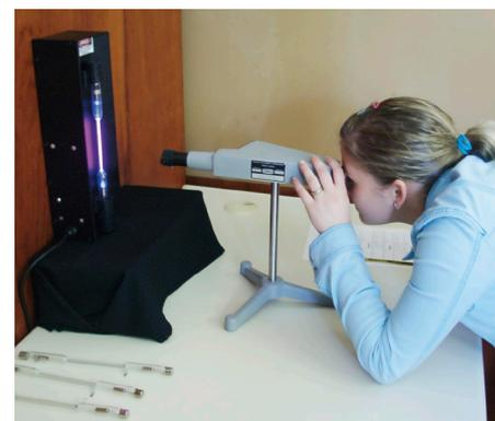
Figure 3. A student uses a spectrometer to observe the spectrum of a gas-discharge lamp. Credit: Ricardo Cardoso Reis.
