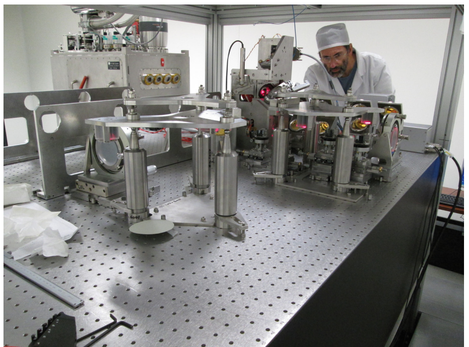
Figure 5. Some views from the laboratories: 5a: A view of some of the components of the cold optics bench, including the beam-shaper box presented in front of the COB backbone; 5b: A discussion concerning the cool-down procedure; 5c: Two of the three electronics cabinets; 5d: Both cryostats
