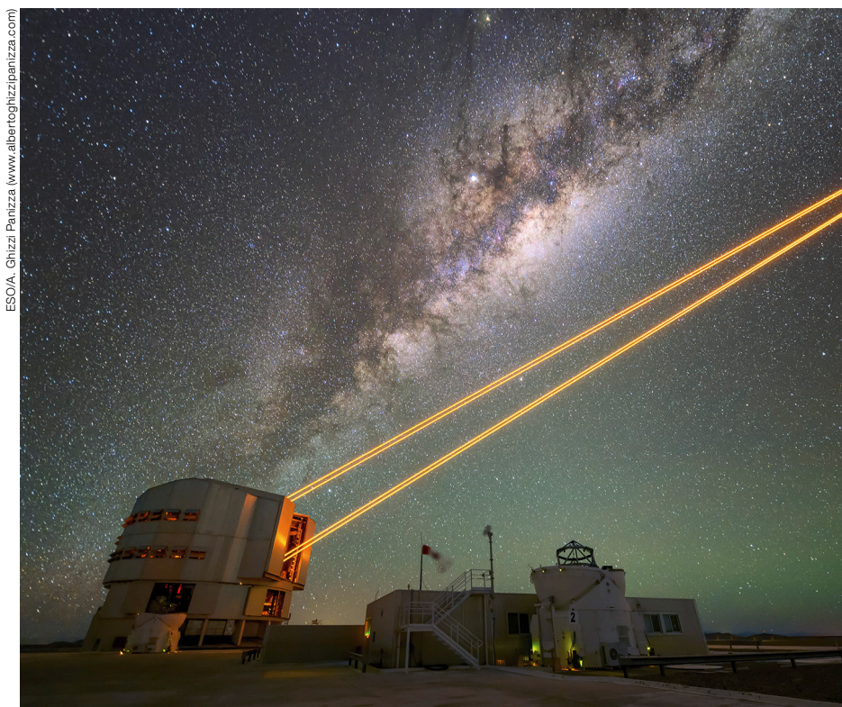
This picture of the week shows four powerful laser beams leaving Unit Telescope 4, or “Yepun”, at ESO’s Very Large Telescope (VLT) in Chile’s Atacama desert. These form the VLT’s 4 Laser Guide Star Facility, which enables astronomers to take extremely crisp images of the cosmos by employing a technology known as adaptive optics.
