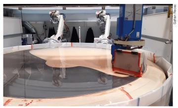
Figure 4. The M3 mirror during the second grinding run.
