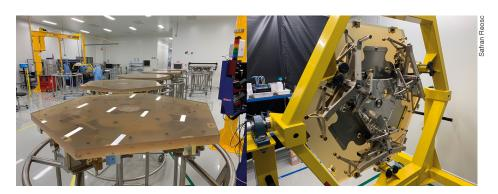
Figure 1. M1 segment polishing at Safran. Left: the segments are waiting for final inspection.
