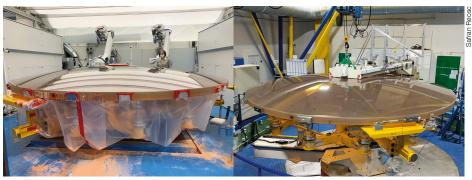
Figure 2. The M2 mirror after its last polishing run: left, on the polishing stand and right, during interferometric measurement
