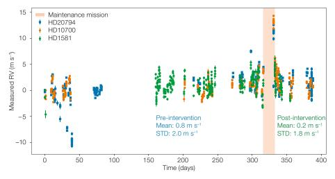
Figure 3. Radial velocity variation of a sample of quiet stars used for instrument stability monitoring. Within the scatter of the measurements no discontinuity is visible in the radial velocities after the completion of the mission.
