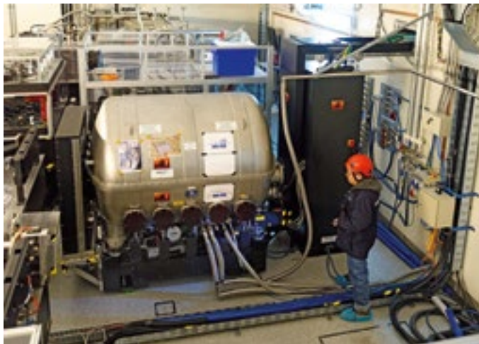
Figure 6. The GRAVITY beam combiner freshly installed in the VLTI Laboratory.
