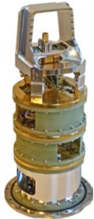
Figure 1. An assembled ALMA Band 5 receiver cartridge, shown courtesy of NOVA/GARD.
