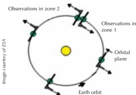
CoRoT is pointed in the same direction for more than 150 days at a time, before the Earth's movement around the Sun leads to the unwanted effect of the Sun's rays entering the telescope. CoRoT then turns 180 degrees around its long axis and points in the other direction
