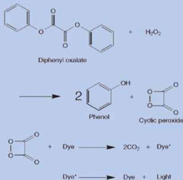
Figure 4: How a glow stick works
