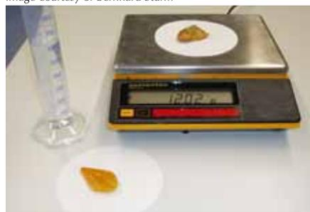
Amber (in front) and flint (on the balance) can be distinguished by determining their density
