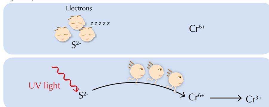
**Figure 6:** Electrons involved in a redox reaction cannot move spontaneously from one reactant to another. UV light supplies the electrons belonging to sulphide ions (the form of sulphur thought to be involved in the darkening reaction) with sufficient energy for them to become mobile enough to be transferred to Cr(VI)
