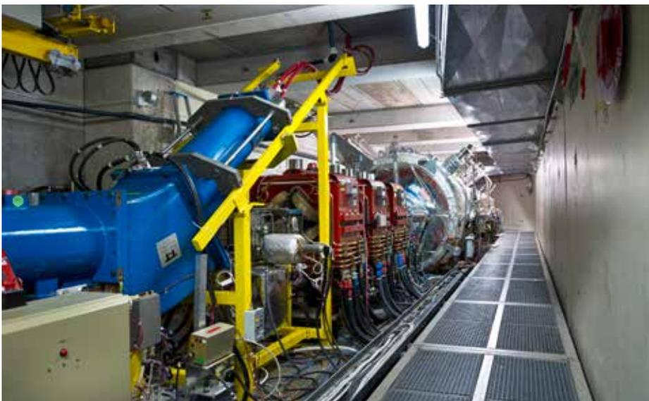
The antiproton decelerator at CERN decelerates antiprotons before sending them to several experiments studying antimatter.
