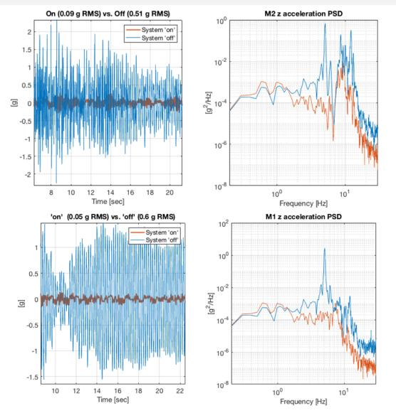
Accelerations M2 z: system 'off' and 'on'
