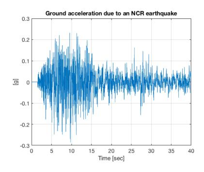
Ground acceleration in Z direction due to a NCR earthquake
