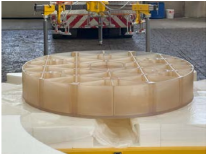
The lightweighted M5 Zerodur blank being packaged for transportation from SCHOTT to GIL
