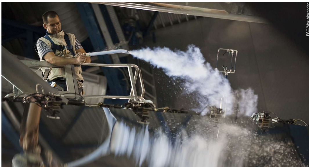
Cleaning mirrors with CO 2 .
