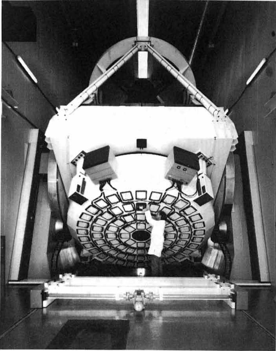
Figure 7.12: **The NTT mirror support system.** The 3.58-m main mirror of the ESO New Technology Telescope (NTT) rests on 78 “active” supports which are controlled by a computer. The system is referred to as “active optics” and was first developed at ESO for the NTT. In this view from below the main mirror, the arrangement of the support compartments in four concentric circles is seen. (PR 03/90: NTT image C04).
