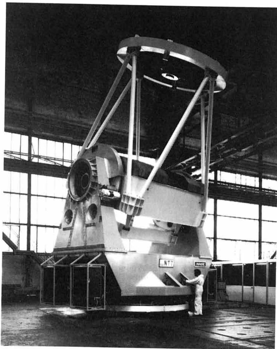
Figure 7.2: **The ESO New Technology Telescope (NTT)** at INNSE in Brescia, Italy in mid-August 1987. This telescope, which incorporates the latest innovations in telescope design, will be erected at La Silla in mid-1988 and is expected to enter into operation before the end of 1988. The mirror diameter is 3.58 m. (PR 01/88; Colour)
