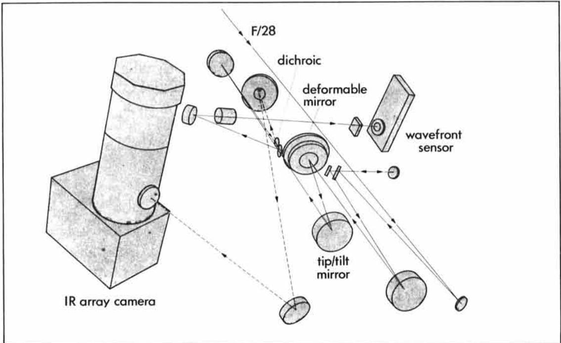
Figure 9.2: **The VLT Adaptive Optics Prototype System.** The picture shows the VLT Adaptive Optics Prototype System, installed during the first test at the coude focus of the 1.52 m telescope at the Observatoire de Haute Provence (France). The light from a star enters the system from the top. The round element at the centre is the deformable mirror. The wavefront sensor is in the upper right part of the instrument. The large vessel at the left houses the cooled, infrared camera. (PR 06/89; BW)
