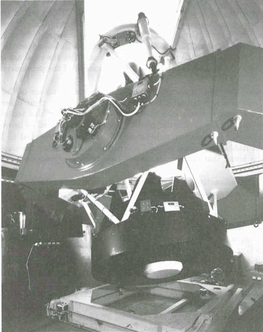
Figure 1.1: The **ESO Coudé Auxiliary Telescope (CAT)** has a 1.4 m primary mirror and is alt-alt mounted. It is housed in a smaller dome, adjacent to the 3.6 m telescope and feeds the 3.6 m Coudé Echelle Spectrometer through a light tunnel. The CAT is fully computer controlled. It has been used for many different types of astronomical observations, including millimetre radio mapping of CO clouds near the galactic centre. (PR 10/87; Colour)
