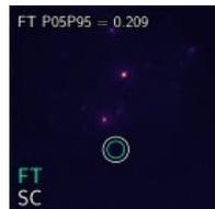
Fig. 9: the position of the science and fringe tracking object has been wrongly picked up
