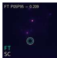
Fig. 8: the position of the science and fringe tracking object has been wrongly picked up
