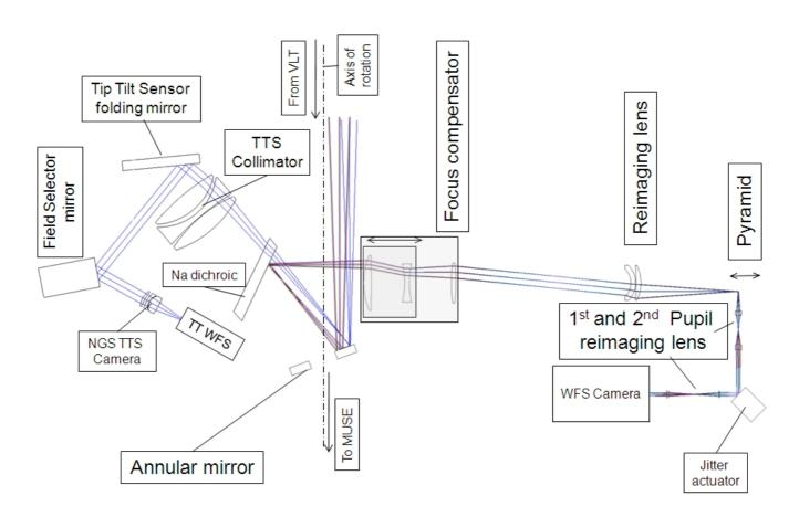
Figure 13: GALACSI WFM layout of the optical paths to the tip-tilt sensor and to one of the LGS wavefront sensor. The MUSE science beam runs unaffected along the axis of rotation.
