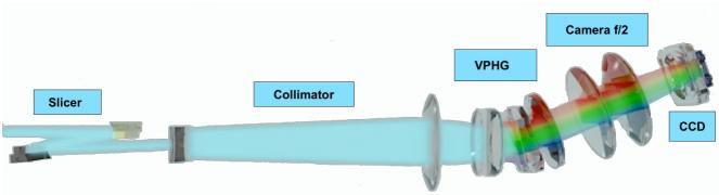
**Figure 7:** Overview of the optical layout for one of the IFUs. The top panel shows one of the slicers, which cuts the FOV of each channel into 4 stacks of 12 slices. The bottom panel shows the optical elements in the IFU and the path of light to the CCD.
