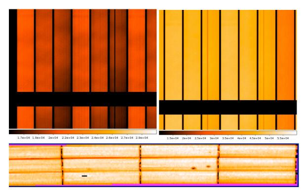
**Figure 20:** Dark features in the MUSE flat fields due to dust in the field splitter. Top: the regions of low transmission extend the full length of the spectrum. On the left is an N-mode flat and on the right is an E-mode flat. Bottom: the 'spots' of low transmission in a reconstructed datacube.
