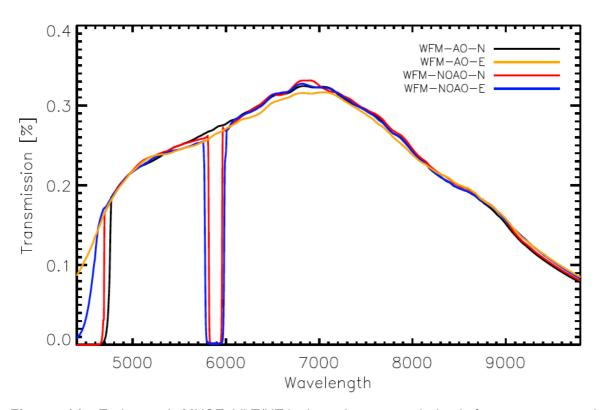
**Figure 14:** End-to-end MUSE+VLT/UT4 throughput, as derived from spectroscopic standard observations.
