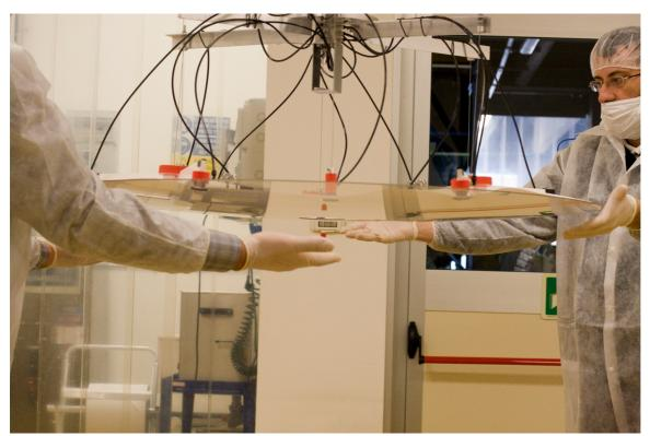
Figure 11: careful handling of the DSM 1.95mm thin shell during manufacturing.
