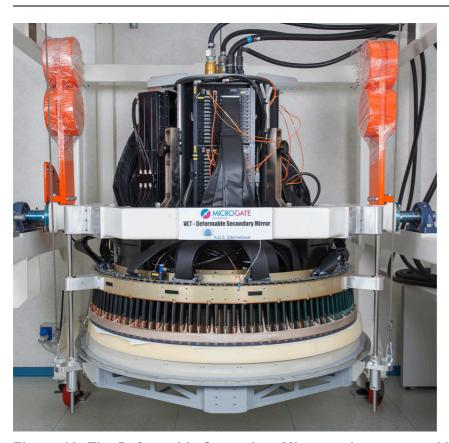
Figure 10: The Deformable Secondary Mirror on its test stand before shipping to Paranal.
