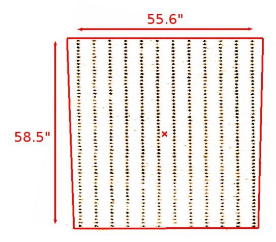
**Figure 23:** Arrangement of the WFM\_SMP mask used for geometrical calibration, as viewed on a reconstructed image when illuminated with internal lamps. We overlay the trapezoidal shape of the FOV in red.
