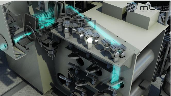
**Figure 6:** 3D view of optical paths for all channels due to the relay optics splitting of the field-of-view into 24 channels. The bottom figure shows the path of light rays for one of the channels, as seen from the Fore-Optics.
