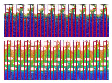
Figure 17: Second order effect in nominal (top panel) and extended (bottom panel) modes, shown here for a bright exposure with arc lines. The red boxes mark the slice limits up to 930 nm. The impact of second order is visible as the white ellipses illuminating the top of the detector. The nominal instrument mode not affected is contamination, but it is more significant in the extended instrument mode.
