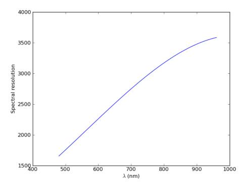
**Figure 15:** Spectral resolution achieved as a function of wavelength, as measured in the lab using calibration lamps.
