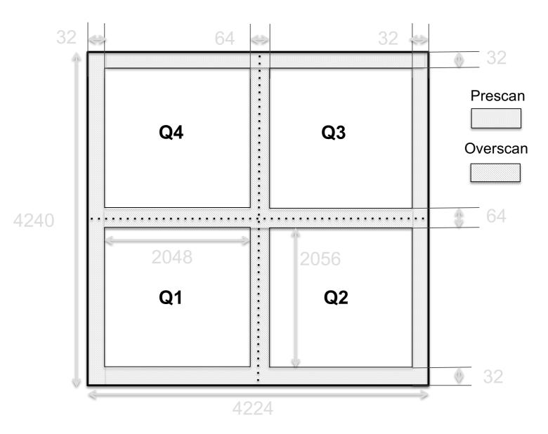
**Figure 8:** Overview of the pixel map of one for one of the detector, showing the 4 quadrants and the pre-scan / over-scan regions. All scales are given in pixels.
