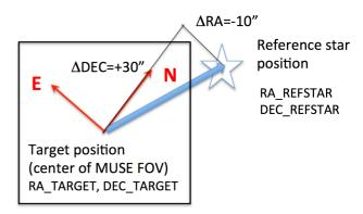
Figure 21: Convention for blind offsets during acquisition.
