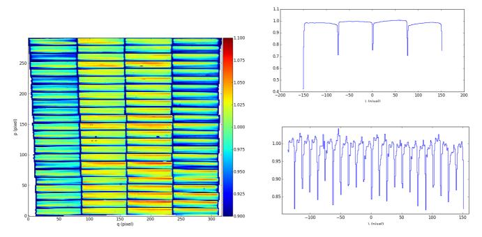
**Figure 16:** (left) normalized reconstructed image of the continuum flat-field in WFM. (right) horizontal (top) and vertical (bottom) cuts through the normalized image showing the horizontal and vertical variations in illumination.
