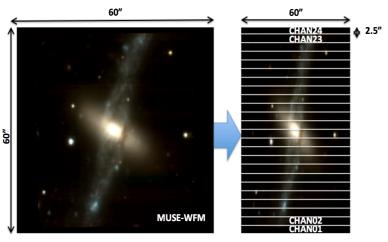
**Figure 9:** Overview of the splitting of the field-of-view from the fore-optics to one of the MUSE detectors. Left: splitting of the MUSE FOV into 24 sub-fields entering each channel. Center: shape of the entrance slicer on sky, with 4 stacks of 12 slices (numbered in red from 1 to 48) covering a 2.5 x 60" field. Bottom: location of each slice on the detector, with the corresponding wavelength range.
